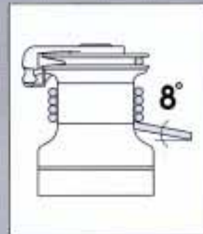
Sheet entry angle must be at least 8°.
