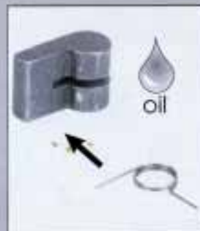
Insert spring with straight leg against pawl. Use oil for lubrication.
