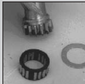
Clean all parts, except 37383 and 37339, with solvent.
