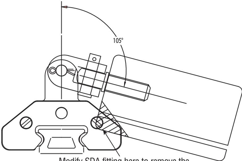
Modify SDA fitting here to remove the shaded area to allow fitting to rotate 105°.
